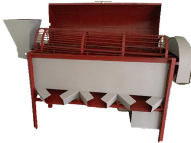
FIGURE 9 Perspective view of the fabricated onion bulb size grading machine
