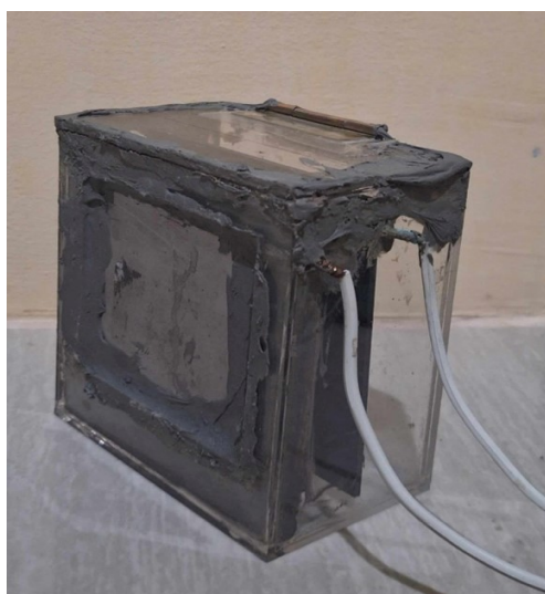
Figure 5. Fabricated Single-Chamber Air-Cathode Membraneless MFC
