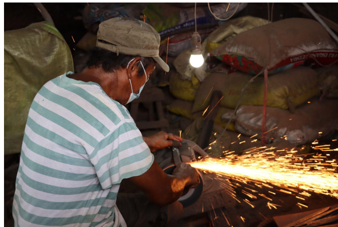
FIGURE 3 The blade is polished to ensure that only a perfect “Tabak” or bolo is produced in the workshop. Photo by Zane Abegail Gonzales.
