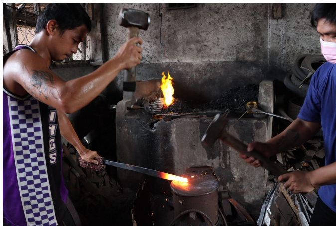
FIGURE 1 Traditional blacksmiths or “panday” alternately hammer on the flaming steel to shape it into a “tabak” or bolo.
