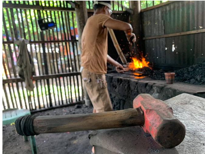
FIGURE 2 The “molye”- a piece of metal scrap is heated in burning coals to soften the steel so that the blacksmith can manipulate and re-shape the steel into its desired.
