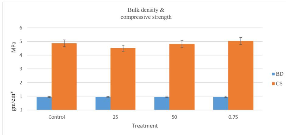
**FIGURE 1** Results of analysis on Bulk density and compressive strength. Compressive strength tested at DOST Taguig, Manila, Philippines in August 2016.
